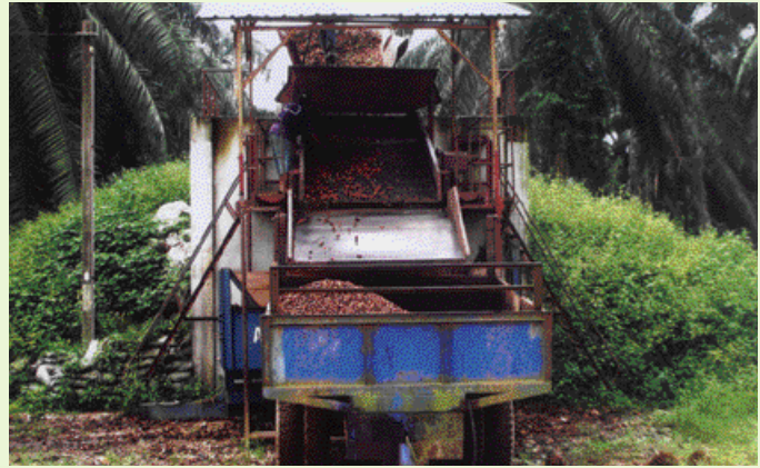
Sifting of loose fruit using the vibrating separator prior to sending to oil mills for processing
