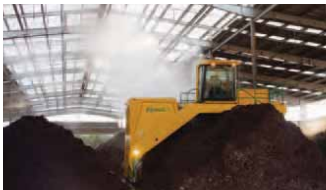
Compost turning to improve aeration and evaporation at Genting Jambongan compost plant
