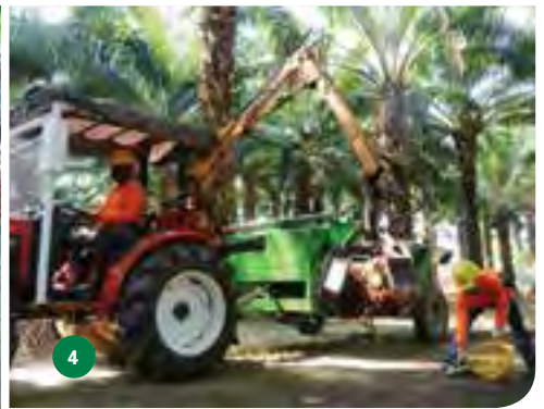
2-4. Implementation of in-field mechanised processes – mini-tractor, crawler, mini-tractor with grabber (left to right)
