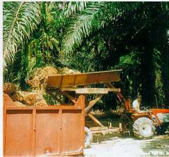
Infield mechanisation practised by the Group. FFB collection using a grabber into the tractor (left). With the use of a scissor lift trailer, the FFB are unloaded into the bin (right).
