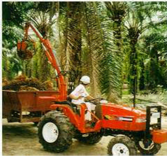
Infield mechanisation practised by the Group. FFB collection using a grabber into the tractor (left). With the use of a scissor lift trailer, the FFB are unloaded into the bin (right).
