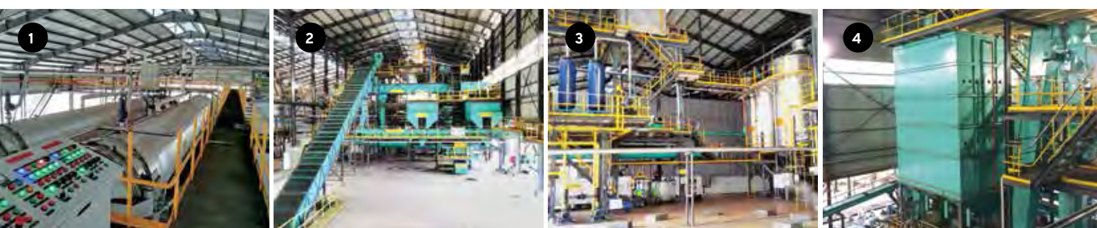
The fully-automated Globalindo Oil Mill is our Group's 3rd oil mill in Indonesia. Automation at various stations at the oil mill - 1. Sterilising station, 2. Threshing station, 3. Clarification station, 4. Kernel station
